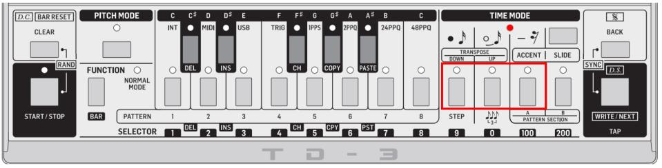
If no timing settings are input, the TD-3 will not make any sound when START/STOP is pressed.
