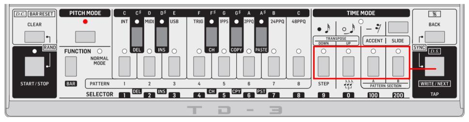
Press PITCH MODE to reset the sequence to Step 1.
